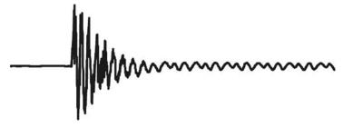
Here is another example of a transient waveform. This is signal of a slapped bass string. In this case, you see a large transient signal that decays to a steady signal.
